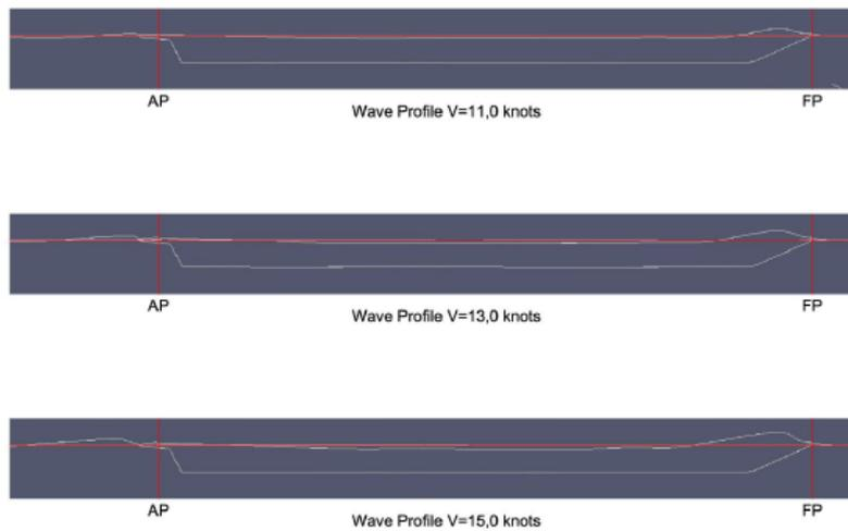
Fig. 5 Plot of the *E-ferry* wave system at 11, 13 and 15 knots
