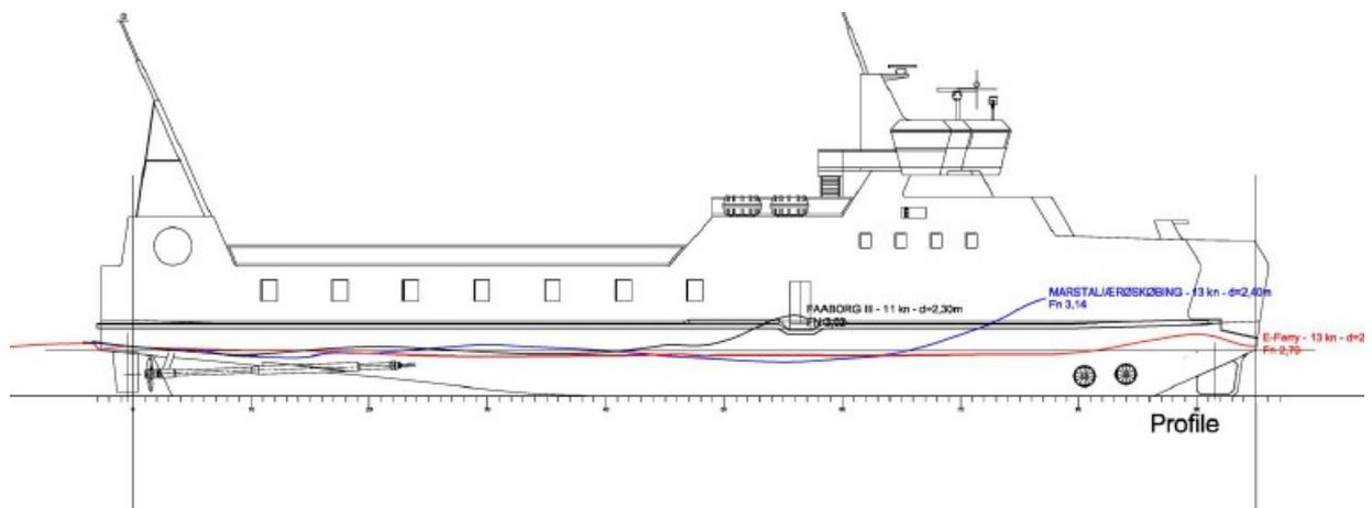
Fig. 6 (a) Plot of the *E-ferry* wave system (at 13 knots) compared with existing, comparable passenger ferries.
