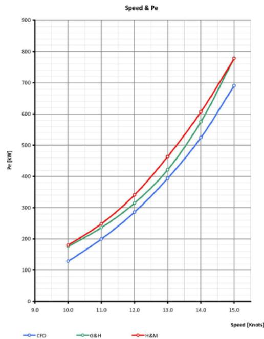
Fig. 6 Hull resistance as effective power from CFD calculations, Guldhammer and Harvald method and Holtrop and Mennen method
