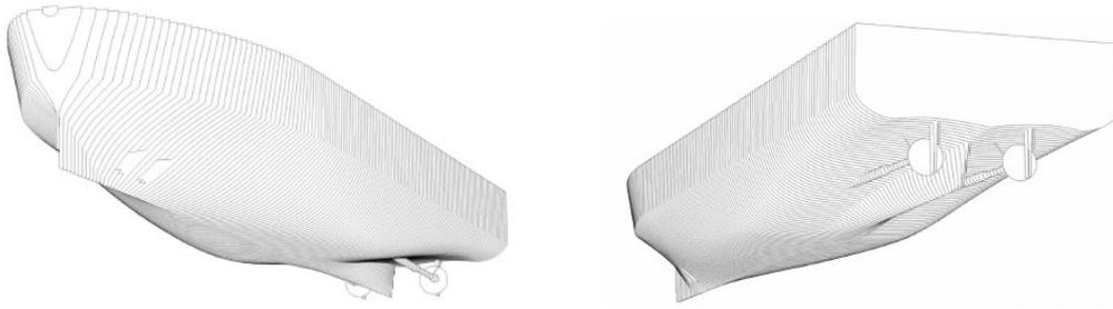
Fig. 4 (a) Plot of the *E-ferry* hull from stem; (b) Plot of the *E-ferry* hull from stern
