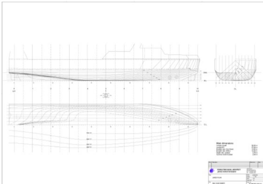
Fig. 3 Line drawings for the *E-ferry* hull
